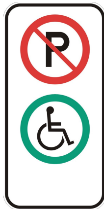
Figure A-3.8.3.9.(2) Sign for barrier-free parking”.
