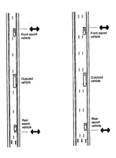
METHOD FOR USING SIGNAL ARROW LIGHTS ON A REAR ESCORT VEHICLES ON A ROAD WITH 2 OR MORE TRAFFIC LANES IN THE DIRECTION TRAVELLED BY THE OUTSIZED VEHICLE
